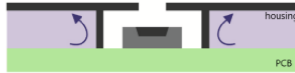
Figure 2. Separating a sensor compartment from the remaining housing minimizes the influence of entrapped air on the sensor.
