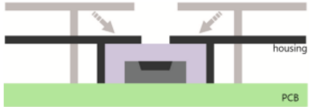
Figure 1. A small dead volume allows for rapid adaption to changes in the environment.
