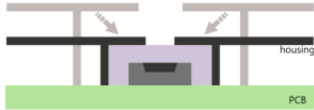
Figure 1. A small dead volume allows for rapid adaptation to changes in the environment.
