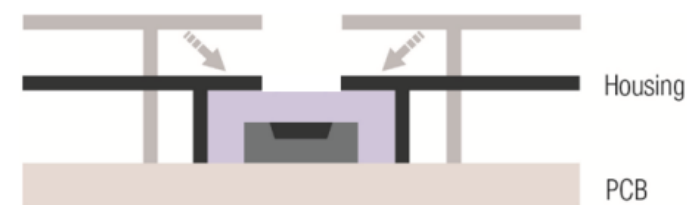
Figure 3: A small dead volume allows for rapid adaption to changes in the environment.
